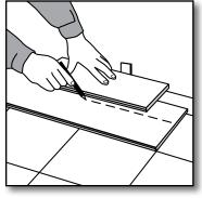
**[11]** Use a full width scrap plank to mark your cutting line on the last row.
