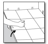
[1] Separate the whole row by carefully lifting up and releasing the whole row. Fold up and release the whole long side of the row, being very careful not to allow the planks to bend downward at the end seams! This could damage the locking mechanism of the plank!
