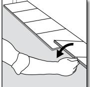
**[3]** Fold down into the locked position with a single movement. The plastic clips will engage to lock this plank into place.
