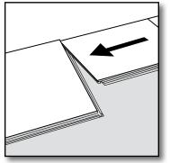
[2] In the first row, place the second plank tight against the short end of the first plank.
