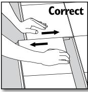
[2] Disassemble the panels by sliding them apart horizontally at the end seams. (Do not fold connected planks upwards!)
