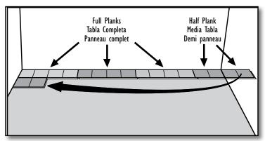
**[6]** Tiles should be the same size at all walls. Start the first row using full planks. Stagger the second row by starting with a half plank for the 12" tile look. For the 16" tile look, stagger the second row by starting with one-third or two-thirds of a plank.
