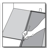
**[4]** Place the final plank face down with the short side (without the locking strip) towards the wall. The remaining expansion space should be at least a minimum of 1/4" from the wall. Draw a pencil line where the plank is to be cut.
