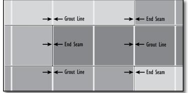
**[7]** The center of each grout line should be used when aligning the grout lines with those of the previous row. This will allow slightly larger or smaller grout widths to appear straight and uniform when viewed across the room.
