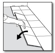
**[8]** Connect the planks in the following rows by aligning the end seam of each plank directly above the end seam of the preceding plank. Insert the long side seam at a slight angle first, and as the top surfaces meet, rotate the plank down into the locked position.
