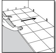
**[9]** The distance to the walls can be adjusted when three rows are completed. Remember to place the flooring a minimum of 1/4" from all walls or other vertical obstructions such as cabinets, pipes, or columns.
